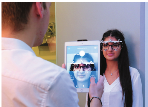
EssilorLuxottica's EyeRuler 2 measures fitting parameters as well as near vision behavior.
